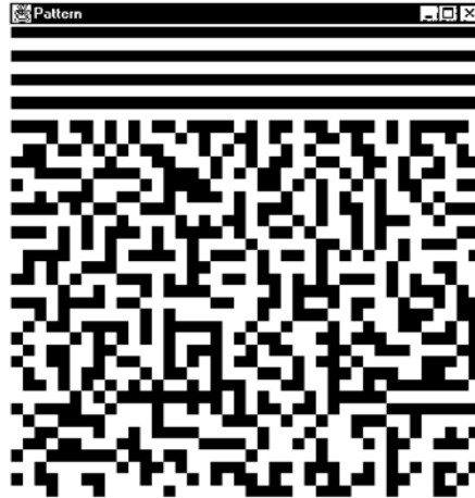
Fig. 8. Generalization-based methodology: a local pattern imposed on a portion of a DCA grid.
